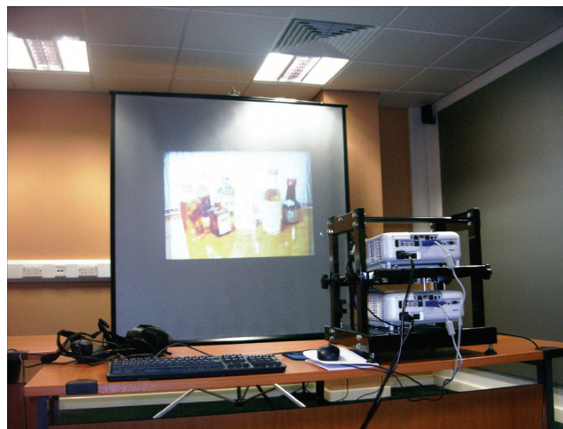
Figure 2: Manchester Computing's portable passive stereoscopic unit, showing 'intoxication' a 3D art piece by Karen Grainger.
