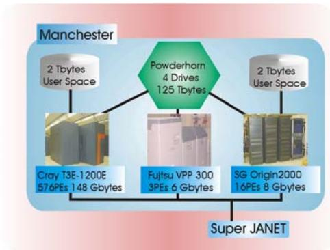
Figure 1: The original machine configuration at CSAR.
